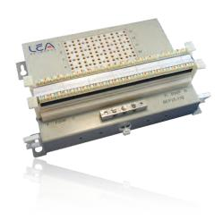
The BEP25-110 consists of a low profile wall mount, epoxy powder coated carbon steel housing, input and output connection blocks, and a high speed data optimized 5 pin modules protection field. An internal 26 AWG fusing wire is included to give maximum isolation in case of catastrophic faults.
