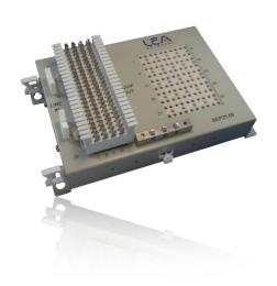
The BEP25-66 consists of a low profile wall mount, epoxy powder coated carbon steel housing, input and output connection blocks, and a high speed data optimized 5 pin modules protection field. An internal 26 AWG fusing wire is included to give maximum isolation in case of catastrophic faults.
