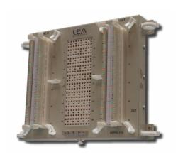
The BEP50-110 consists of a low profile wall mount, epoxy powder coated carbon steel housing, input and output connection blocks, and a high speed data optimized 5 pin modules protection field. An internal 26 AWG fusing wire is included to give maximum isolation in case of catastrophic faults.
