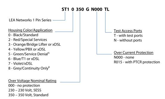
A – "5" types have no electrical connection to equipment, they may be ordered as a grounding module, or with OSP line protection
