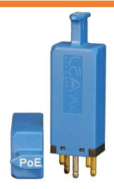
Overvoltage breakdown is nominally 90V, and over current ratings are available at 100mA and 500mA ratings, and are self resetting. Modules are equipped with an internal balanced fail-short mechanism to ensure personnel safety and superior equipment protection in accordance with NFPA, UL and Telcordia requirements.
